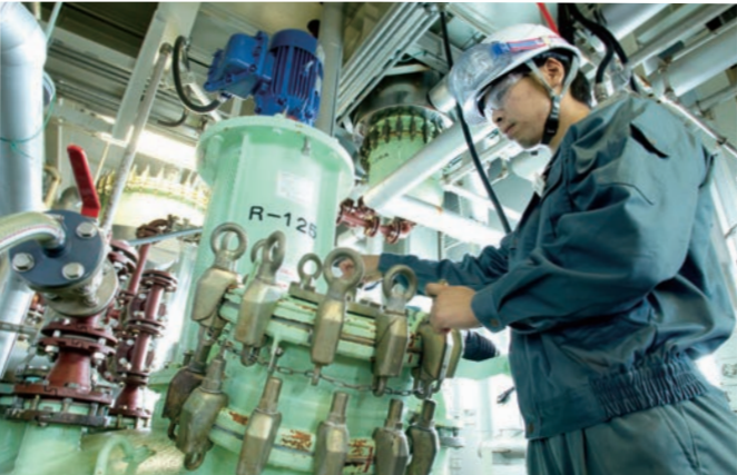
反応缶／Reaction Can 原料を反応させるだけでなく、液体製品の受器、また反応後の処理操作に使用します。 This equipment is used not only to cause reactions of ingredients, but also as a receiver for liquid products and for disposal operations after reactions.
